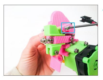
Attach the feeder arm with m3x30 and M3 serrated washer. Do not overtighten. The feeder arm should be able to move.
