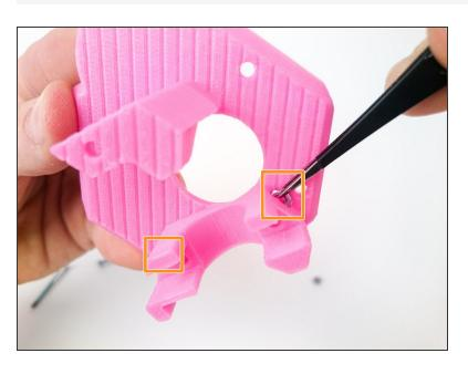
Drop two M3 nuts into slots in the extruder base.
