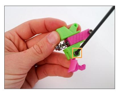
Attach the feeder latch with an M3x14. Do not over tighten.
