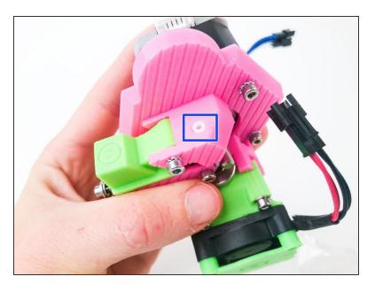
Install the PTFE tube at the top of the extruder.
