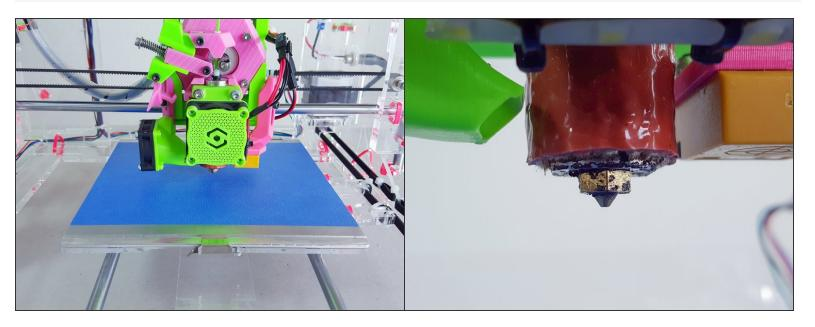
Position the extruder around the middle of the build plate.
