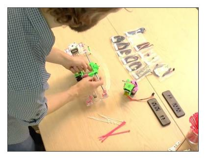
• Pre-install a 4" zip tie with a head out on the right side of the X carriage.
