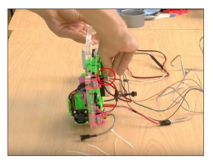
• Connect the wire for the extruder motor to the header on top of the motor.
