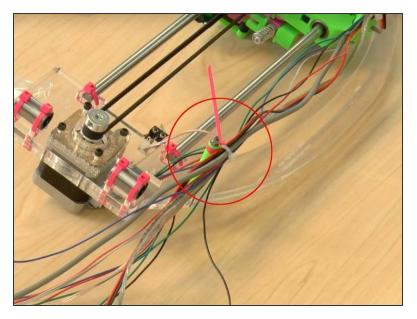
• Use the 4" zip tie attached earlier to form a loose loop around the wires. All the wires must enter the loop from the same direction (from the right in the picture); including the X end stop and X motor wires.
