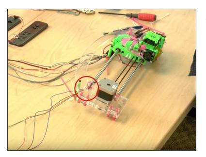
• Above the X motor is a hole in the frame. Thread the x motor wire through it.
