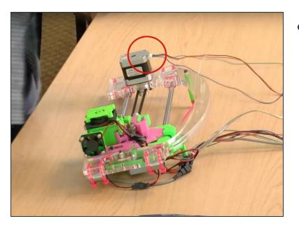
Attach the X motor wire to the header on top of the motor.
