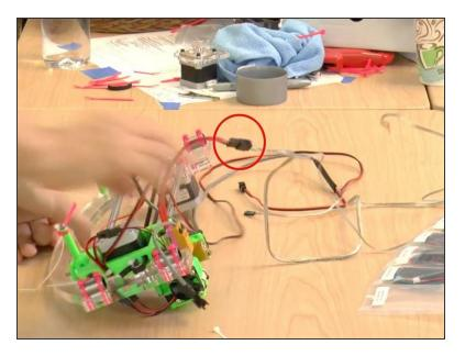
• Connect the heat block and thermistor wire.
