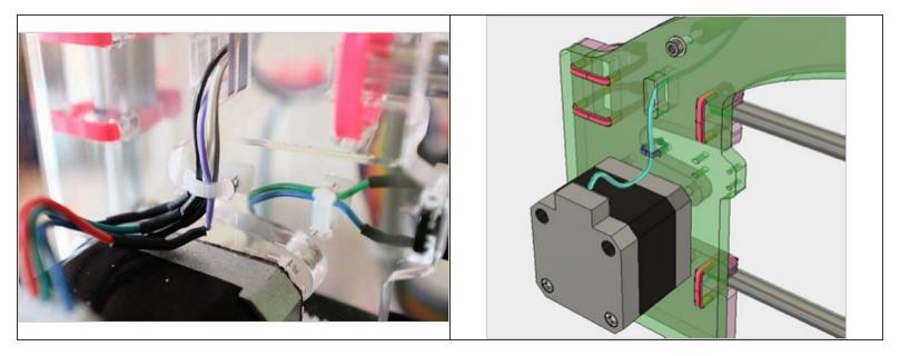
Use a 4" zip tie to secure the X motor wire. Make sure there's plenty of slack in the wire. This will result
