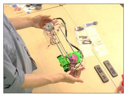
• Use the longer piece of spiral wrap on the rest of the wires. If you're building with a friend this is a good place for a race to see who can wrap the remainder faster.
