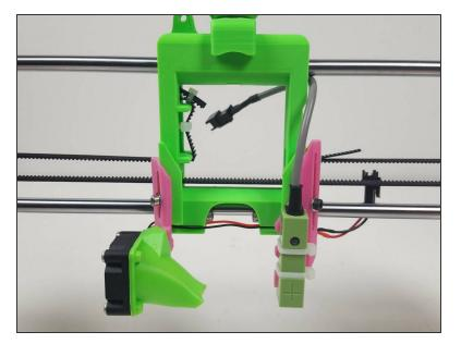
• Done! Both the fan and the sensor are attached to the X-carriage.
