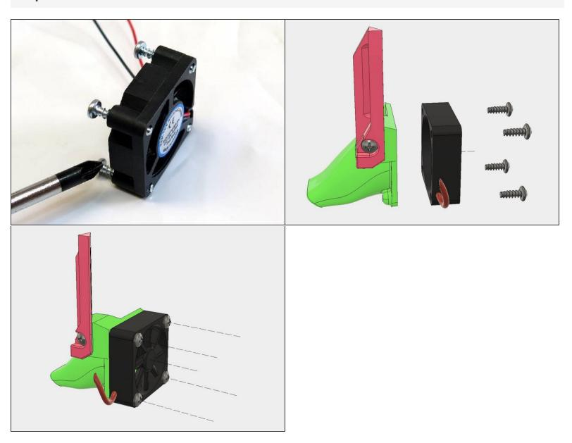
Attach a small 30mm filament fan to the shroud with four plastite screws. Pay attention to the orientation of the fan in reference to the fan cable. Align the fan so that the wires extend to the lower right when looking straight at the shroud.
