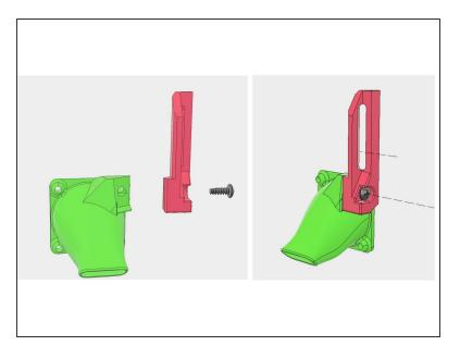
Connect the green filament fan shroud and the pink shroud mount with a single plastite screw.
