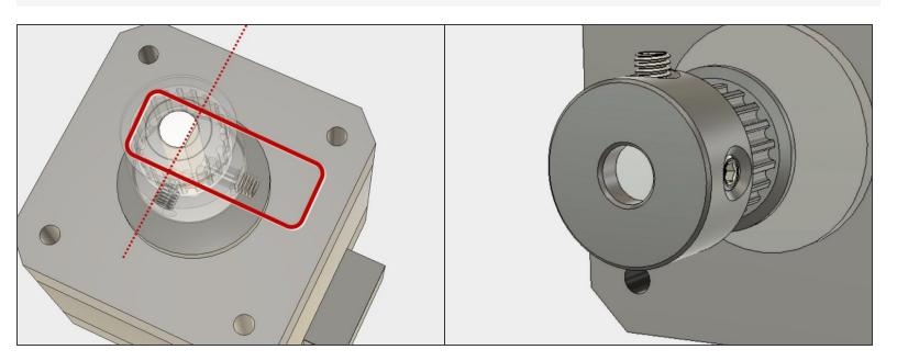
• Tighten as much as you can without damaging the thread (so called 'stripping'). Make sure one of the set screws is against the flat side of the motor shaft. This prevents the pulley from spinning around.
