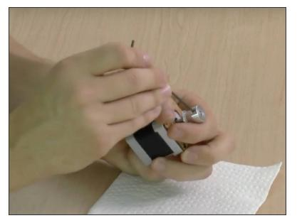
• Slide the pulley as far away from the motor as you can. Yet the set screws should still fully grip the motor shaft. The X pulley will be extending about 3mm (0.12") beyond the top of the X motor shaft.
