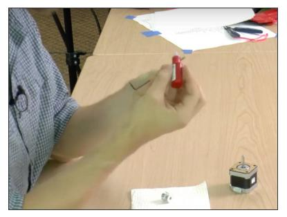
• Same as putting the thread lock onto the Y Pulley set screws. Take out two set screws out of the pulley, put thread lock into their threads, and put them back into the pulley.
