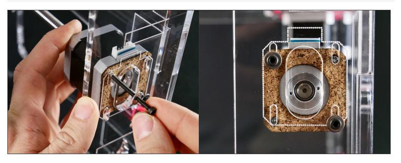
● Keep the screws a bit *loose*. We'll adjust the Z motor position later.
