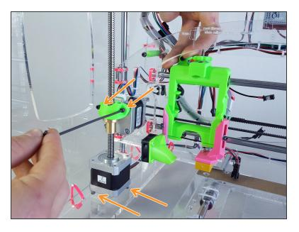
Make sure the ZX coupler and Z motor screws are LOOSE
