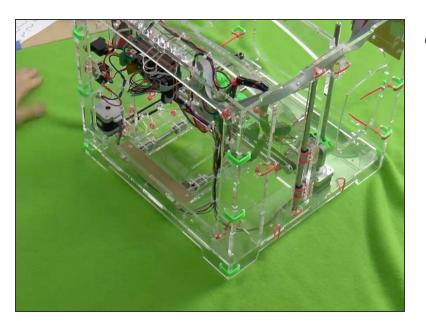
Use the six corner clips to attach the back panel to the box.
