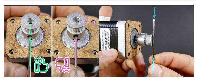
↑ Tighten the longer set screw against the FLAT side of the motor shaft.
