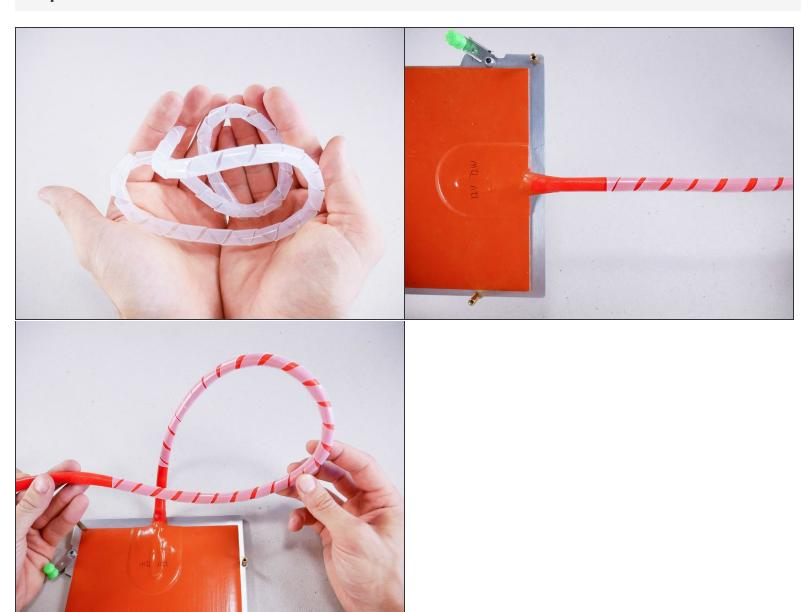
Wrap the wiring in spiral wrap for protection, and you're done!
