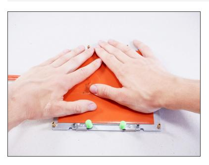
Firmly press the silicone heater pad onto the aluminum base.
