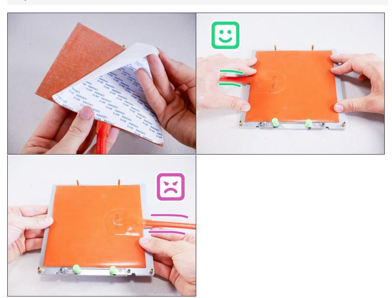
• The heater pad may be slightly larger than the bed. The outside edge is just silicone - you can trim it with a knife after installation.
