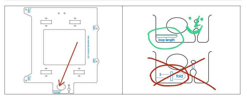
[update] The etchings on the bottom of the Y assembly have changed. Functionally, it's the same.
