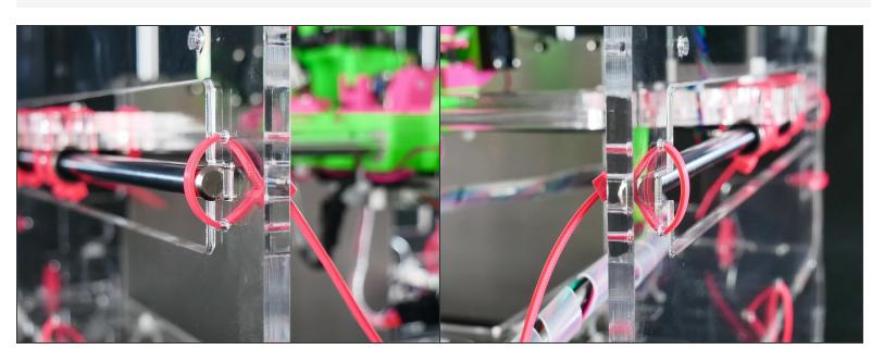
Note that on the **left** the rod is **outside**, while on the **right** the rod is **inside**.
