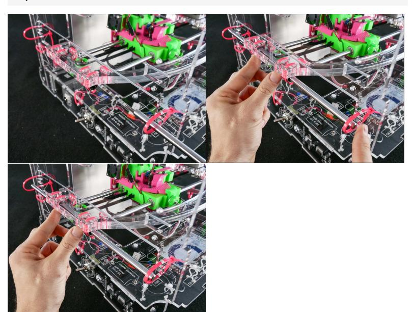
Be gentle. Do no force the rod and keep it straight or you may damage the ball bearing by knocking some balls out.
