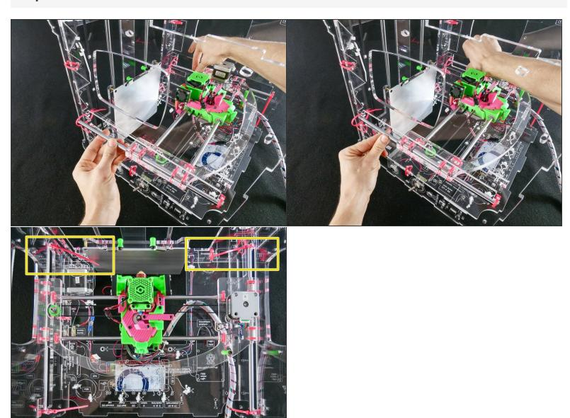
Push the rods in place and tighten the back zip ties.
