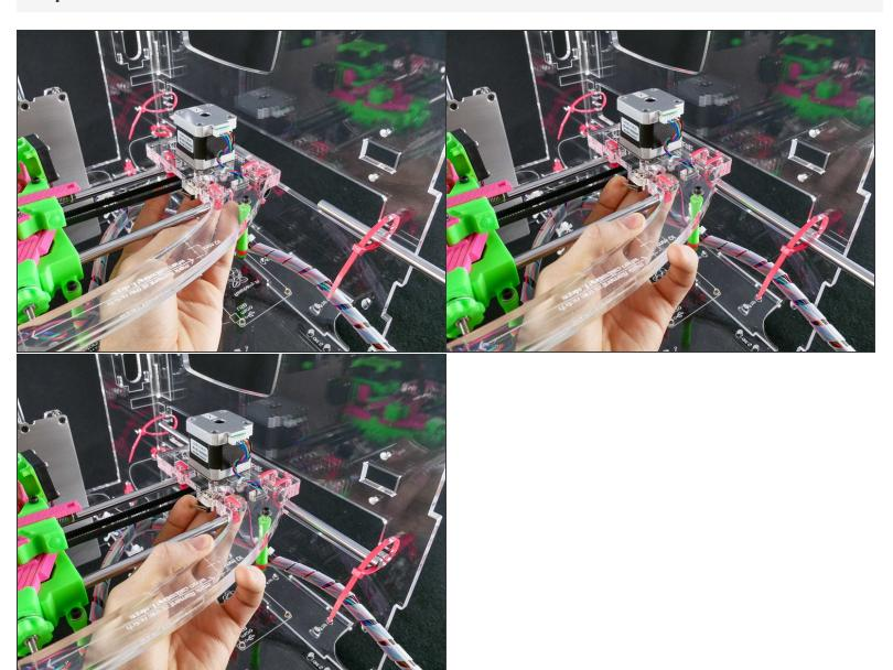
↑ BE GENTLE. Do no force the rod and keep it straight oryou may damage the inside of the bearing.
