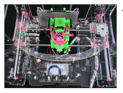
The X assembly is inserted.
