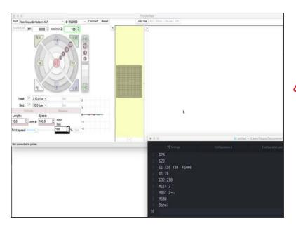
Follow the video walkthrough to find and save the correct z probe offset. Gcodes used in the video follow:
