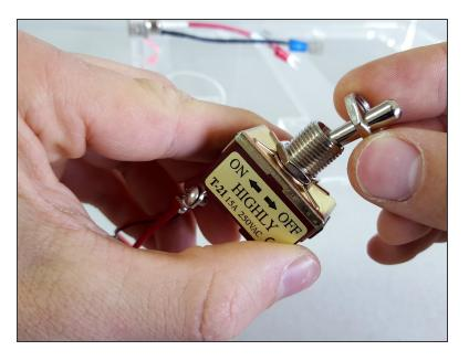
Remove one nut from the front of the power switch.
