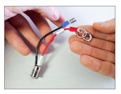
Remove the nut and spring washer from the connector.
