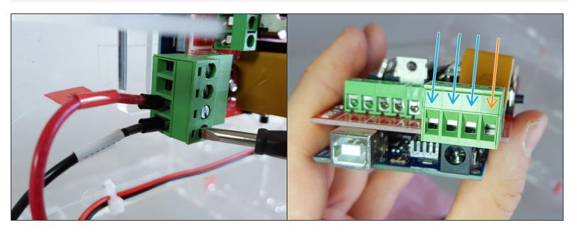
Make sure to properly insert the power wires into the green RAMPS power connector, and tigten them very well. If you leave this connection loose, it may lead to excessive contact oxidation, excessive resistance, and eventually to a melted connector or fire.
