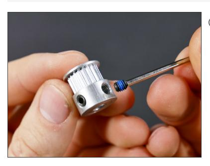
These little things are called set screws or grub screws. Our set screws also have a blue nylon patch that prevents loosening by vibrations (the patches are a kind of threadlock)
