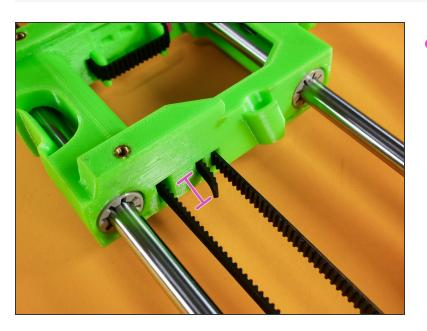
Leave a bit less than a centimeter (3/8 inch) of the x belt intact in case you ever need to disor-re-assembly your JellyBOX.
