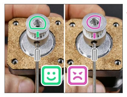
Rotate the pulley so that one **set screw** is against a **flat side** of the motor shaft. This is extremely important.
