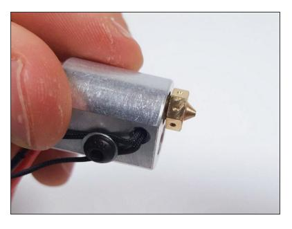
Unscrew the nozzle about 1/2 of a turn (180 degrees) to create a small gap between the nozzle and the heatblock.
