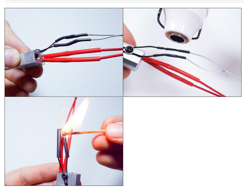
Slide the heatshrink down over the now crushed ferrules and shrink into place with a heat source such as a soldering iron, hot air gun or a flame.
