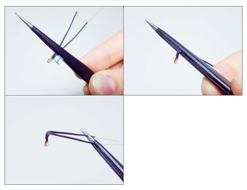
Bend thethermistor legs 90 degrees about 2-3mm behind the glass bead.
