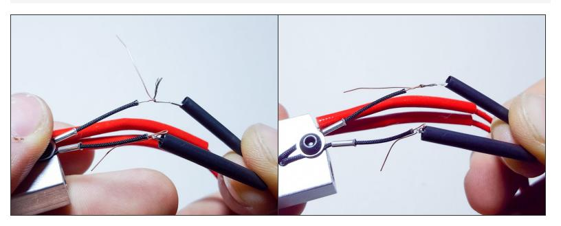
• It does not matter which wire is which. The thermistor does not care about plus and minus.
