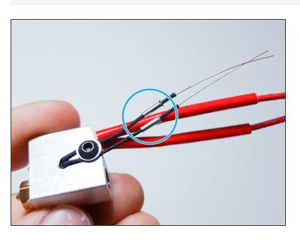
Slide on two ferrules onto the thermistor legs.
