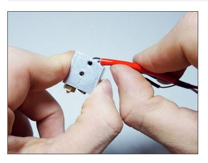
Gently bend the red heat cartridge wires at about 90 degree angle straight back (see picture).
