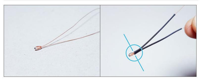
The thermistor is small and fragile. Be gentle with the legs. The thermistor bead is made of glass - don't crush it!
