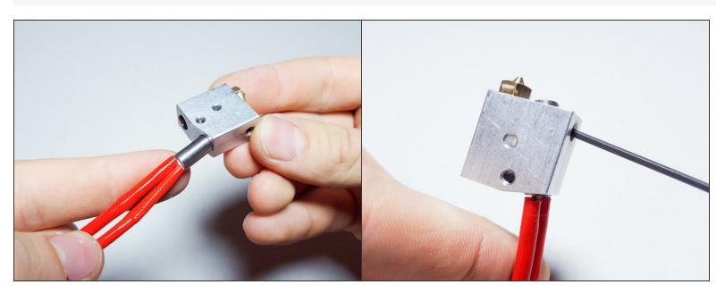
Secure the heater cartridge with an M3 set screw.
