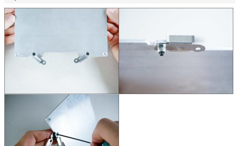
⚠ Leave the screw a bit loose so the clips can swivel.
