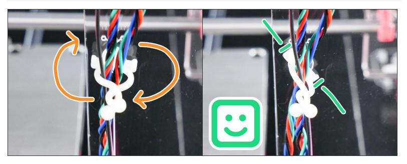
The trick is to rotate the twist locks. This effectively makes their diameter smaller and constrains the wires better.
