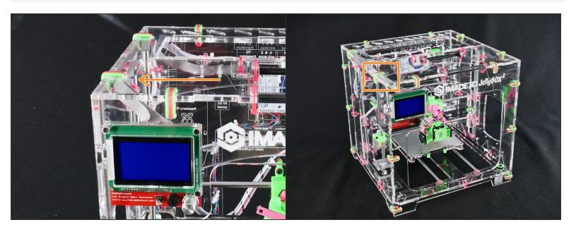
On the top left, the zip ties alsohold the LCD wires in place.
