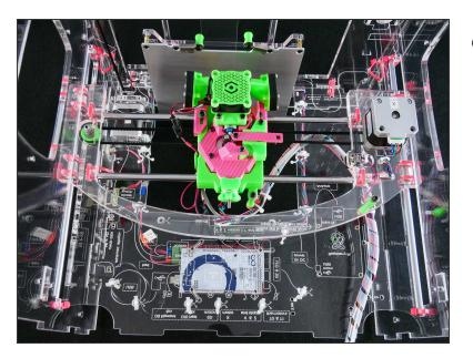
• The X assembly is inserted.
