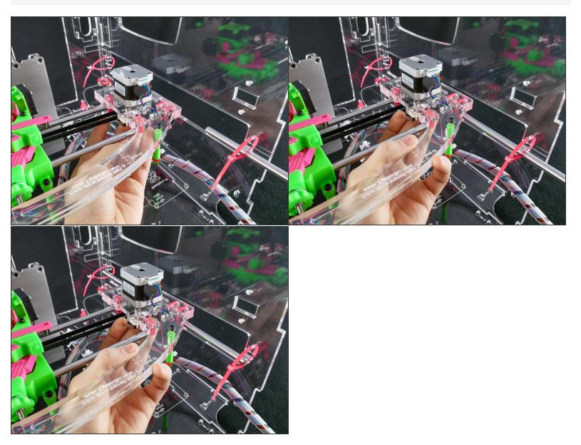
A BE GENTLE. Do no force the rod and keep it straight oryou may damage the inside of the bearing.
