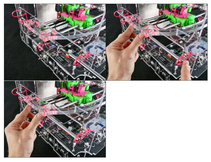
Be gentle. Do no force the rod and keep it straight or*you may damage the ball bearing by knocking some balls out.*
