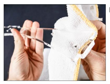
Any dirt and fingerprints trapped between the acrylic parts will be impossible to clean later!
