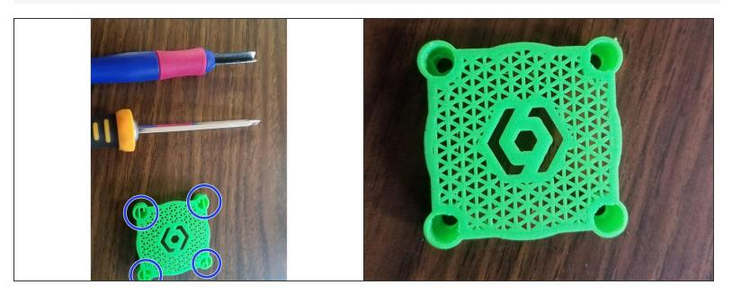
Use a Small Screwdriver and a small circular Blade to Remove the supports from the part and clean any remnants.
