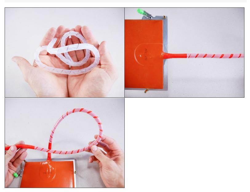
Wrap the wiring in spiral wrap for protection, and you're done!
