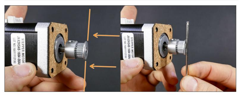
Make the top of the motor shaft**flush** with the top of the pulley.
