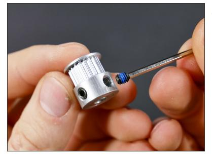
(i) These little things are called **set screws** or **grub screws**. Our set screws also have a *blue nylon patch* that prevents loosening by vibrations (the patches are a kind of *threadlock*)
