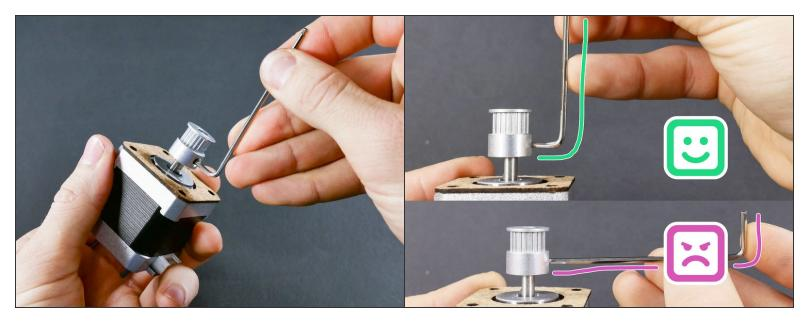
⚠ Tighten both set screws well using the long side of the hex key. We do not want these to be loose.
