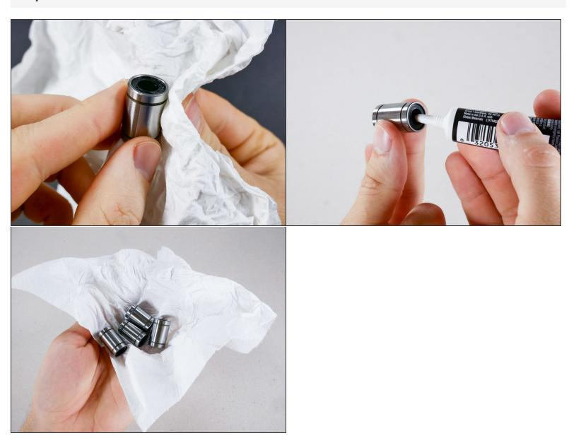
Just like you did with the Y bearings, put a drop of oil into the X bearings.
