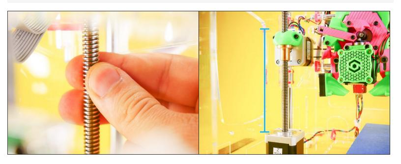
• Rotate the Z rod to move the whole X assembly about this high.
