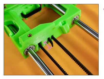
Leave a bit less than a centimeter (3/8 inch) of the x belt intact in case you ever need to disor-re-assembly your JellyBOX.
