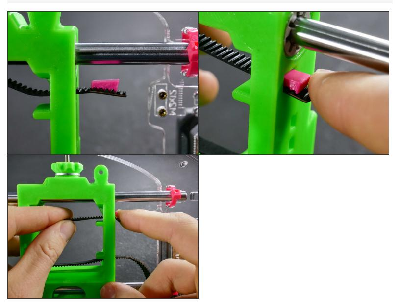
• The position of the wedge on the belt is not precise - you only need to make sure to dit the belt teeth into the wedge teeth.
