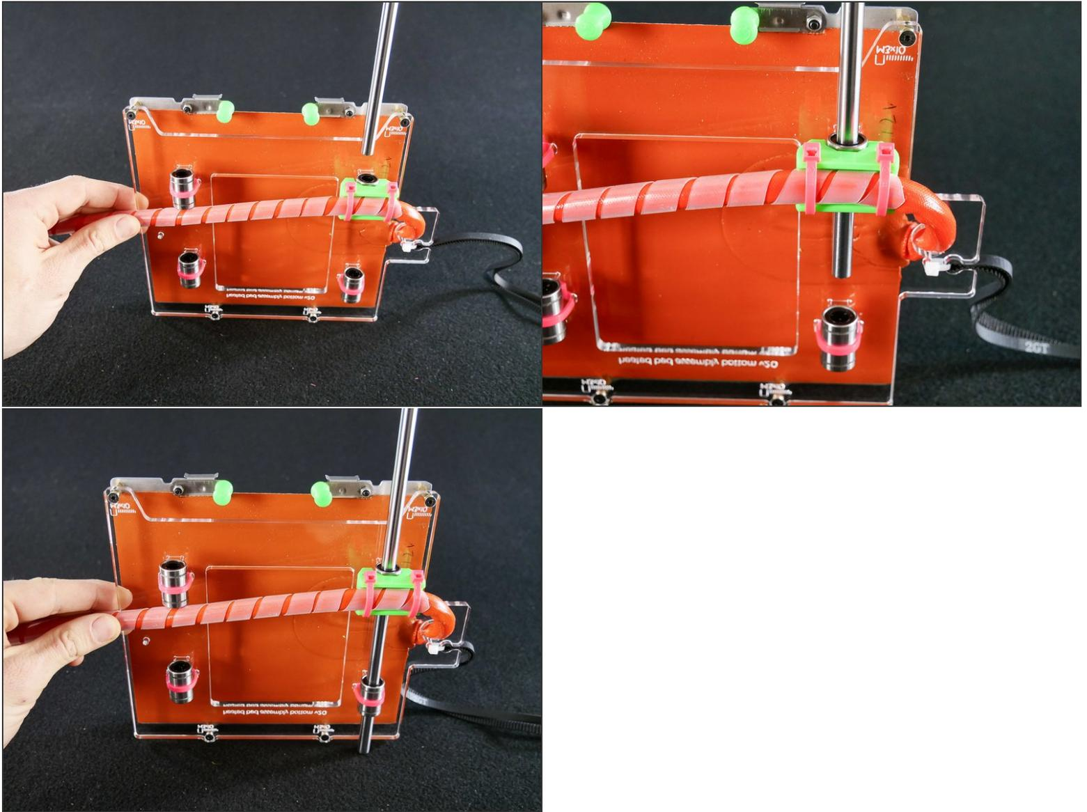
**⚠ Be gentle.** Do not force the rods and keep them straight or you may damage the ball bearing by knocking some balls out.
