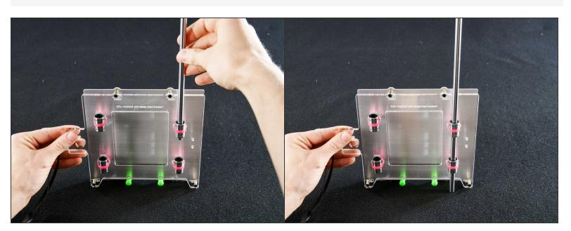
Be **gentle**. Do no force the rods and keep them straight or you may damage the ball bearing by knocking some balls out.
