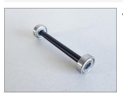
Pre-install the bearings onto the rods.
