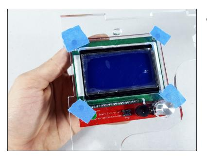
• Optional: hold the screws in place with a bit of (blue) tape.
