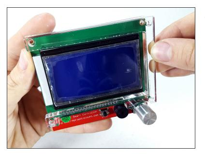
• Align the **6mm** spacer to the front of the controller.
