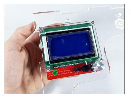
• Attach the LCD controller to the front acrylic piece.
