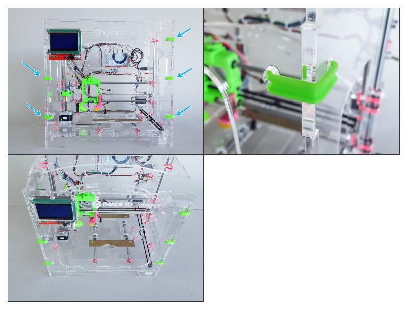
• Slap the front onto the printer and secure with the green corner clips.
