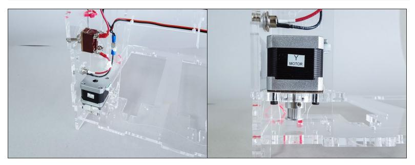
• Snap the Y Motor into place (with the pulley facing down) right under the power supply connector.
