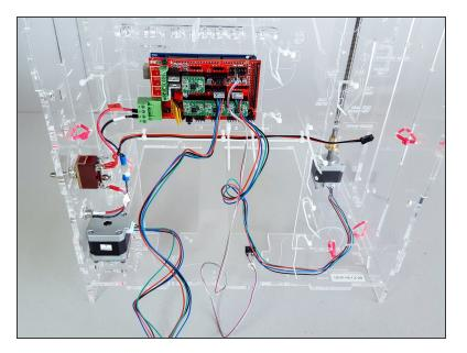
• All connected. It's time to tidy it up the wires.
