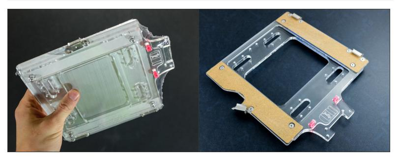
Partially assembled Y axis with the build plate attached.
