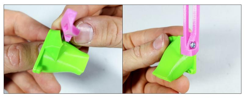
• Connect the shroud and the mount with a plastite screw.
