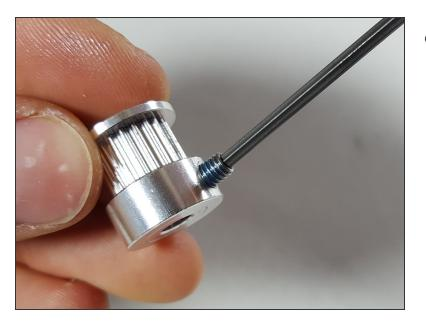
• Re-insert both set screws into the pulley.
