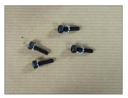
• Put serrated washers onto four M3x12 screws.
